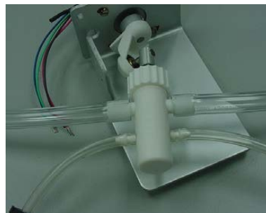
Example of pump with rinse ports at rear of pump (note: hose clamps have been removed for photo clarity).
