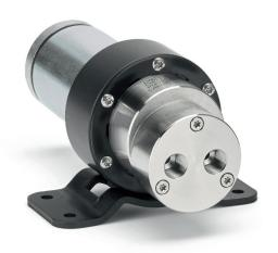
The Optima series is designed for applications requireing a very small package size. The construction is the same as those of it's larger cousins, but by removing one of the shaft bearings the overall length is much shorter. The inlet and outlet ports can be located on the side or end of the pump, and are available in a variety of sizes. The brushstyle DC motor is oversized and gives excellent brush life at optimum price-performance-ratio.
