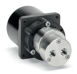
The Optima series is designed for applications requireing a very small package size. The construction is the same as those of it's larger cousins, but by removing one of the shaft bearings the overall length is much shorter. The inlet and outlet ports can be located on the side or end of the pump, and are available in a variety of sizes. The brush-less DC motor has an integral flange allowing bulkhead mounting, and its IP-55 rating ensures it will stand up to harsh environments.
